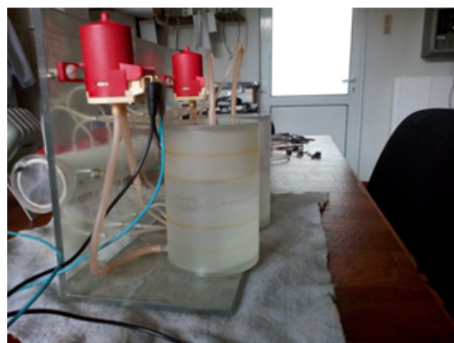
Fig. 2. Micellar ultrafiltration device (view)
